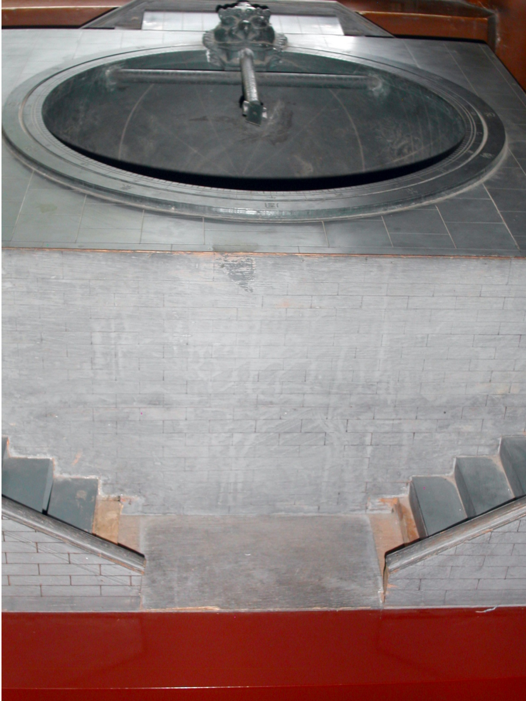
Figure 7. Model of Up-facing Instrument designed by Guo to measure the position of the Sun and progress of solar eclipses.
