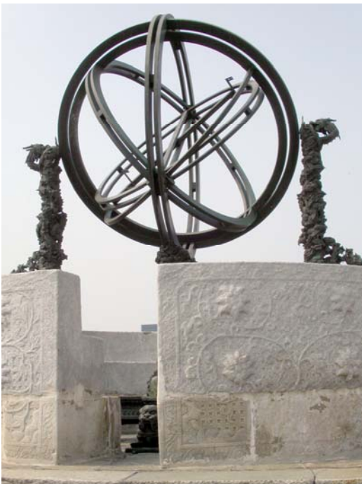
Figure 5. Example of a more complex armillary sphere built in 1744 AD with interlaced dials for measuring time and celestial positions.
