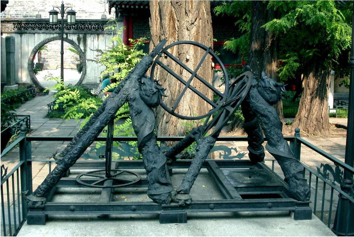
Figure 4. Model of Simplified Instrument, an armilla designed by Guo c.1280 AD to measure positions of celestial bodies.
