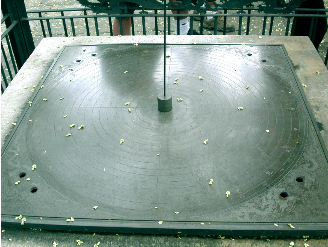
Figure 6. Reproduction of Square Table designed by Guo to gauge angles along the horizon, or azimuths.
